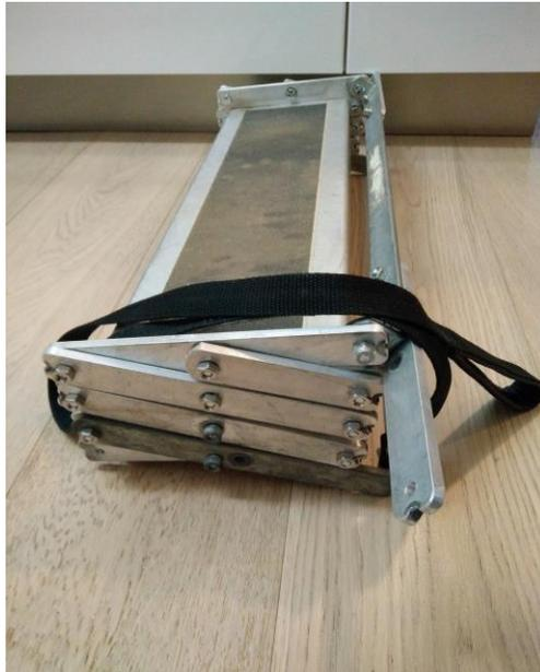
Figure 1. ChairStairs in fully retracted position.
