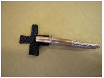
6. Apply a dot of hot glue on the end of the tubing that the foam will be placed and let dry. This rounds the tip of the tubing so that the copper will not cut through the foam and scratch the screen or track pad it is being used on.
