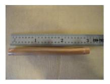
2. Solder 4 lines about 1 3/8 inches long along the end that will not be covered in foam. Before soldering, make sure to clean the copper by rubbing it with fine sand paper and wiping it down with rubbing alcohol. This holds the tip steadier when it is inserted into the headstick.
