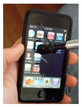
After a couple of tests which included sanding the end of the headstick and covering a wooden ball with conductive material, Geoff recommended that we try using conductive foam that we had in our electronics workshop. The foam worked well. We determined that the surface area of the foam touching the screen was important for reliable operation. We experimentally determined that 3/8-inch diameter works, but is not completely reliable, while ½-inch diameter works reliably.
