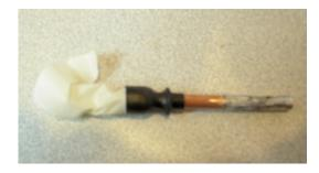
11. Let the Plasti Dip dry and then remove the tape. Below are pictures of the finished product in the headstick. Also there are pictures of it being used on an iPod Touch 2G and you can see that the user is switching pages on the home screen to see more icons.
