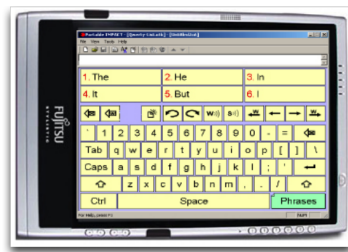
Impact Word Predictor / Fujitsu touch tablet used by AAC speaker
